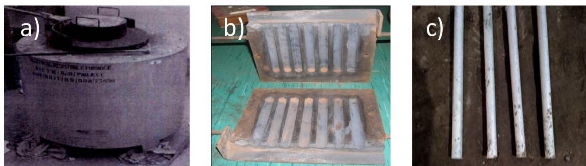
Figure 1 (a) External view of electrical resistance furnace, (b) Metallic dies with 18 mm diameter and 170 mm height for the casting of cylindrical fingers, (c) Castings Obtained
