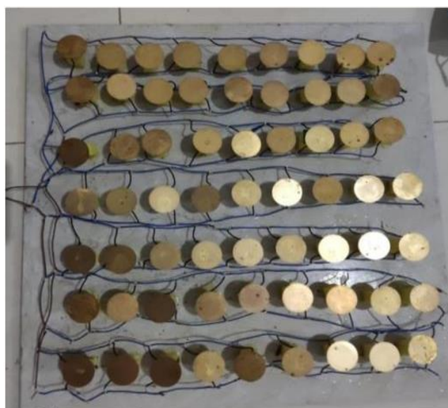
Figure 10. Parallel circuit of piezoelectric transducer
